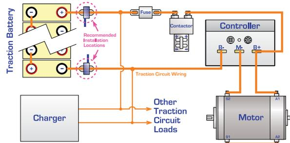
The flow of conventional current (+ve to -ve) should go from the back to the front of the current sensor – that is, the side with the mounting bracket should be oriented towards the positive terminal.
