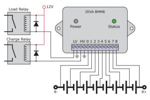
Follow a similar schematic when using multiple modules monitoring packs larger than 8 cells. SSR outputs are isolated so may be wired in series, and can be used for either directly switching power relays, or to signal external master control units.
