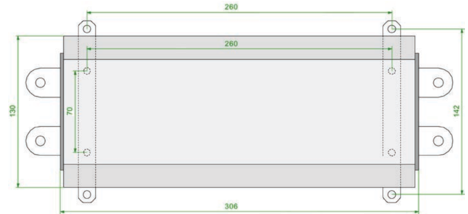
Controller dimensions and mount locations
