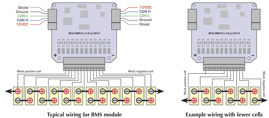
The CAN plugs are Molex C-Grid SL type. They are designed for fairly small gauge wire, around 22-30AWG. The wire's insulation needs to be small enough to fit into the plug housing, which limits outer diameter to about 2mm. The best way to connect wires to pins is crimping first then adding a little solder to the joint. A suitable crimping tool is available from vendors such as Altronics (part T1537).
